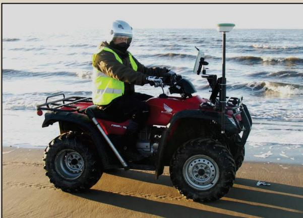
Beach topographic survey undertaken atv mounted GNSS
