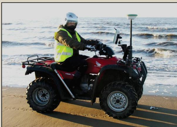
Beach topographic survey undertaken atv mounted GNSS
